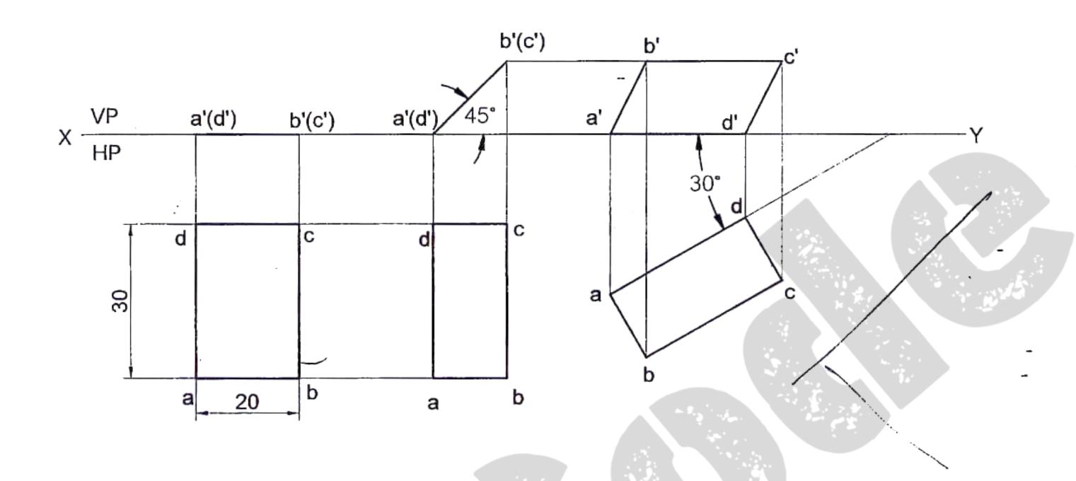
Problem 13 A rectangular lamina of 35mm x 20mm rests on HP on one of its shorter edges. The lamina is rotated about the edge on which it rests till it appears as a square in the top view. The edge on which the lamina rests being parallel to both HP and VP. Draw its projections and find its inclinations to HP and VP.
