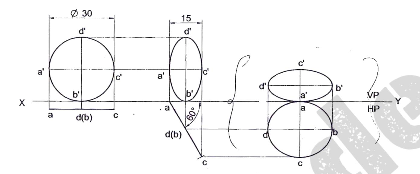
**Problem 50** A circular lamina of 30mm diameter rests on VP such that one of its diameters is inclined at 30° to VP and 45° to HP. Draw its top and front views in this position. **Solution**
