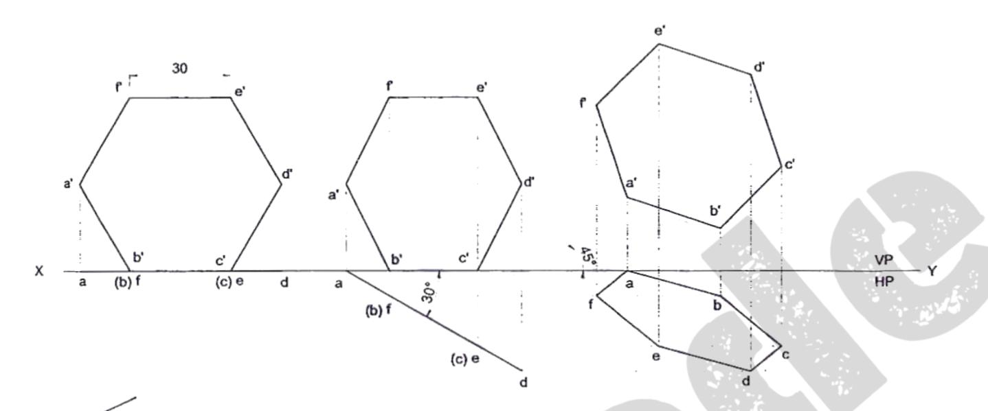
Problem 40 A hexagonal lamina of sides 25mm rests on one of its sides on HP. The lamina makes 45° to HP and the side on which it rests makes 30° to VP. Draw its projections.
