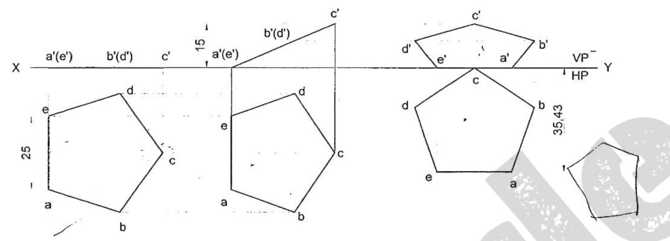
**Problem 23** A pentagonal lamina having edges 25mm is placed on one of its corners on HP such that the perpendicular bisector of the edge passing through the corner on which the lamina rests is inclined at 30° to HP and 45° VP. Draw the top and front views of the lamina.
