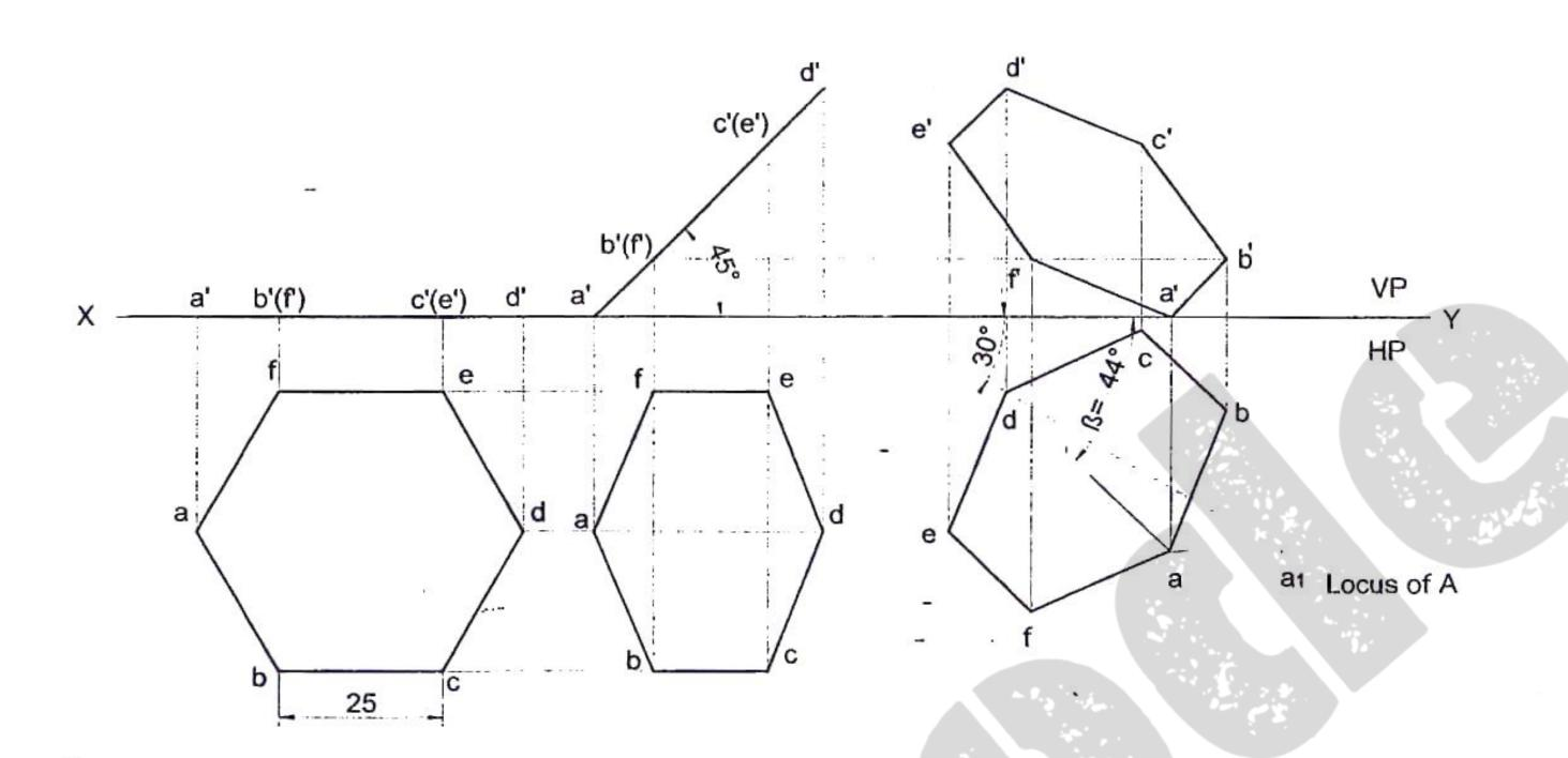
Problem 42 A hexagonal lamina of sides 25mm rests on one of its corners on HP. The lamina makes 45° to HP and the diagonal passing through the corner on which it rests appears to be inclined at 30° to VP. Draw its projections. Solution
