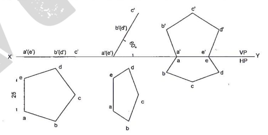
**Problem 25** A pentagonal lamina of sides 25mm is having a side both on HP and VP. The surface of the lamina is inclined at an angle of 60° with HP. Draw the top and front views of the lamina.
