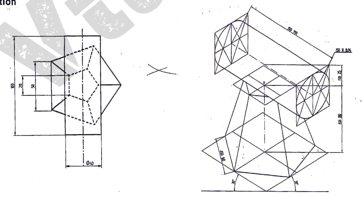
Problem 5 Following figure shows the front view of combination of solids consisting a cut sphere and frustums of a cone and a square pyramid. Draw the Isometric projection of the combination of solids.
