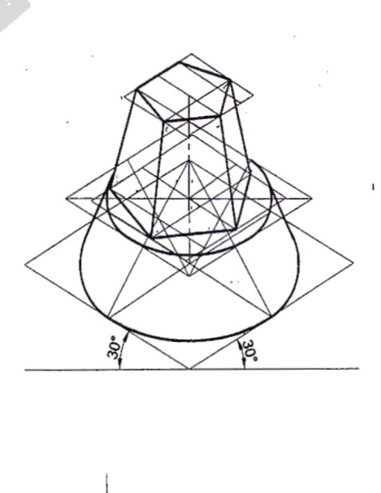
Problem 17 A cone of base diameter 50mm and height 40mm is placed centrally on the top face of a square slab side-80mm and height20mm. Draw the isometric projection of the combination
