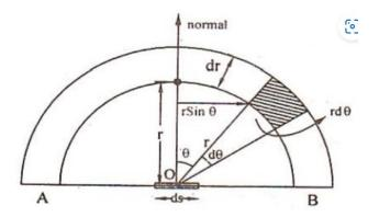
consider a small element 'ds' on a plane wall AB. Assume that the element ds receive the sound energy 'E'.
