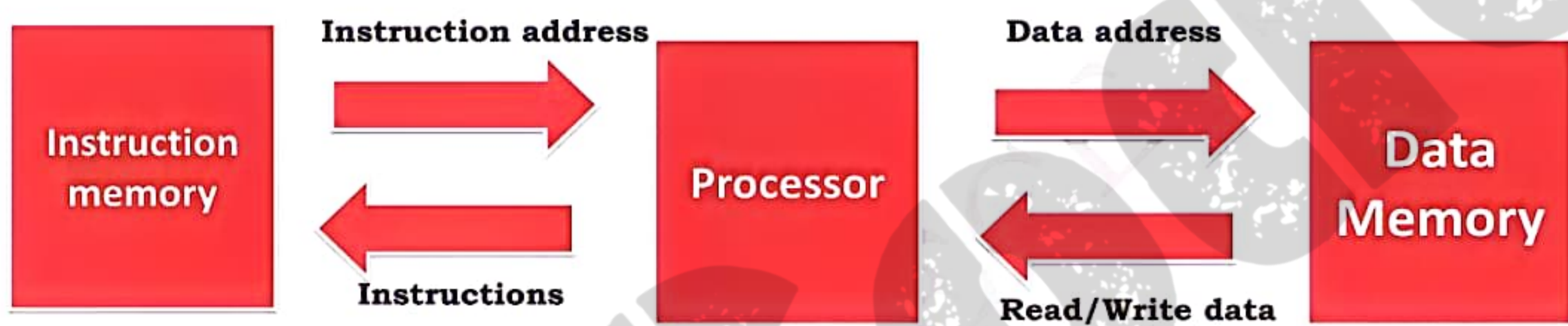
Fig: Von Neumann Architecture with separate memory for instructions and data
