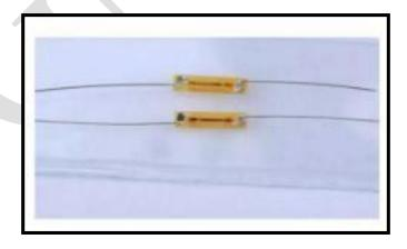
**8. Photoelectric Strain gauge** The photoelectric gauge uses a light beam, two fine gratings, and a photocell detector to generate an electrical current that is proportional to strain. The gauge length of these devices can be as short as 1/16 inch, but they are costly and delicate.
